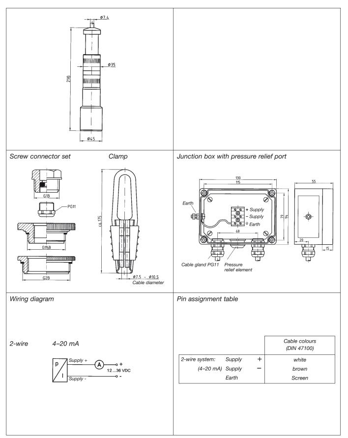
The units are supplied with a detailed wiring diagram.
